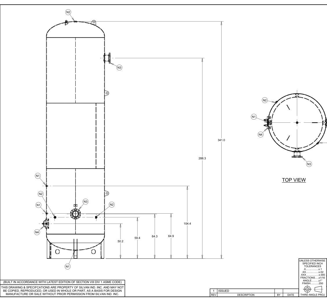
NOZZLE CHART NOZZLE ID NPS SIZE TYPE N1 NPT N2 NPT N3 300# FLG N4 12 X16 MANWAY 300#
